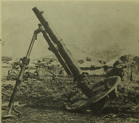
A Russian 120-mm mortar captured by UN troops in Korea from the Chinese and North Korean communists. The Russians recognized the importance, and made full and effective use, of big guns in the last war against Germany. Artillery will play the same indispensable and vital role in any future war.
