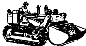
Drott Skid-Shovel on International Crawler. Lift Capacity from 3,000 to 9,000 pounds, 4 models. Digs, fills, rolls back, transports, raises, loads.
