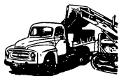
R-164 Series, International Dump Truck. Gross Vehicle Weight, 17,000 pounds; Body dimensions in inches: 108x78x15. Proved steel-flex frame. Wide variety of trucks and dump bodies available.
