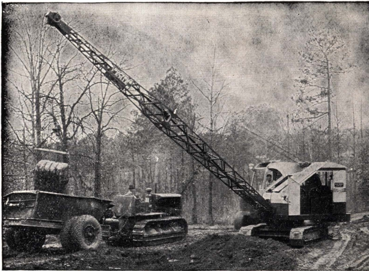
Equipment similar to this will soon be in operation at the Mindanao Mining Company. Bucyrus-Erie Manufactures the machine, which is the new 19-B 5/8 yard power shovel.
