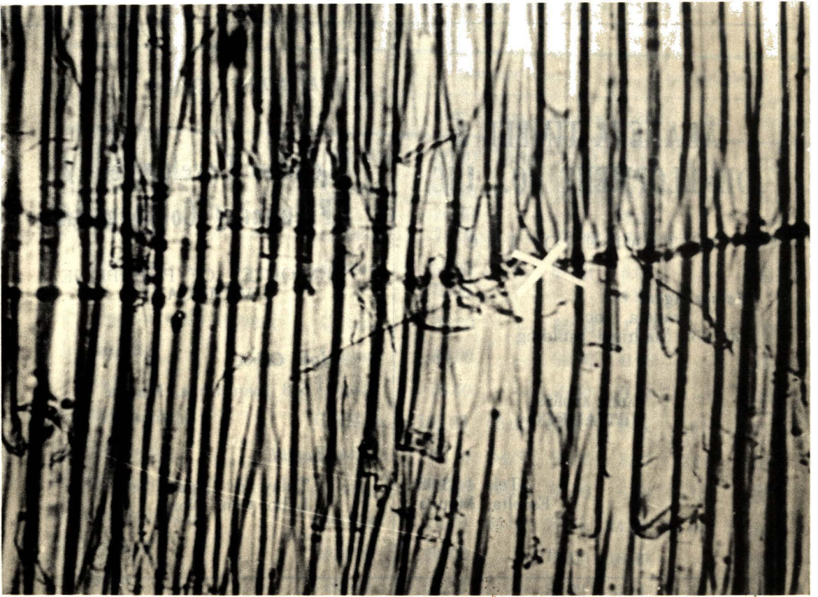
FIG. 1. — Radial section of tangile (Shorea polysperma (Blanco) Merr.) showing the minute compression failures as evidence of a brash wood or brittleheart.
