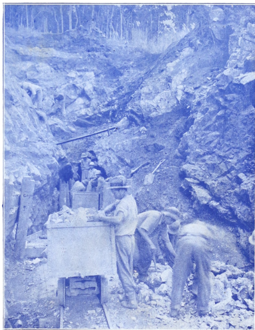
Ore Cars loaded with highgrade chromite at Florannie Mines as shown in the picture, are dumped by ship's hoist into steamers loading at the company's docks. It is a Benguet Consolidated operation.
