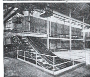
Two Link-Belt flight conveyors handle raw sugar to pivoted overlapping bucket carrier.
