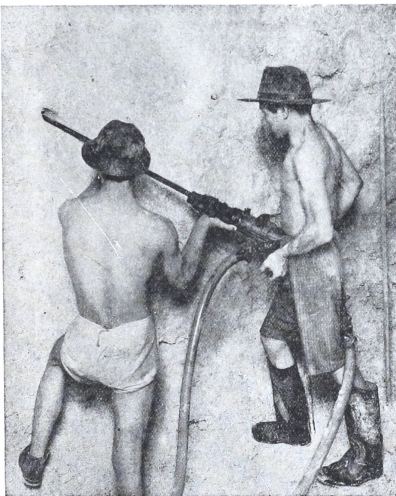
Ingersoll-Rand Jackhammer in use at Benguet Consolidated Mng. Co. Photo by Merl La Voy
