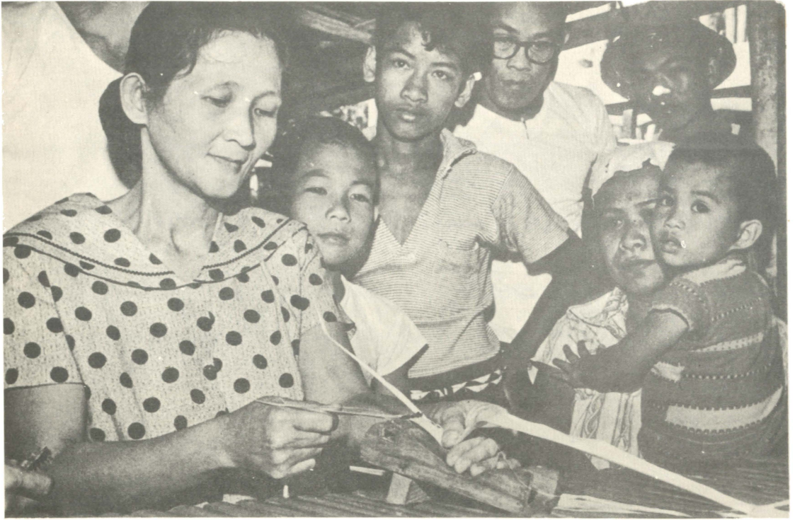
A layer of malabuh bast is passed through a crude wooden block with protruding blades known as "agpang", dividing the strips smoothly and equally.
