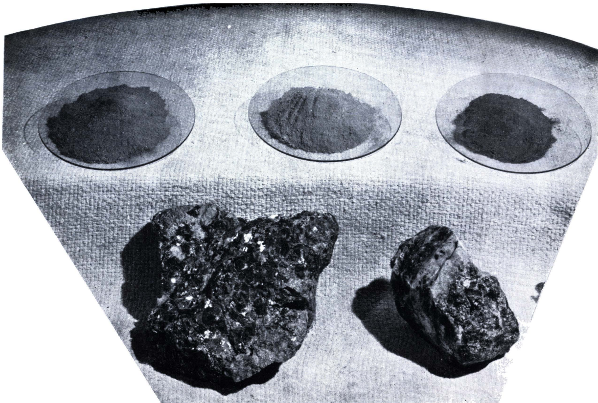
From these concentrates and ores come the gold and silver: top row, left to right, flotation concentrates from United Paracale, San Mauricio, and North Camarines. Bottom row, high grade direct smelting ores from San Mauricio and from Santa Barbara.
