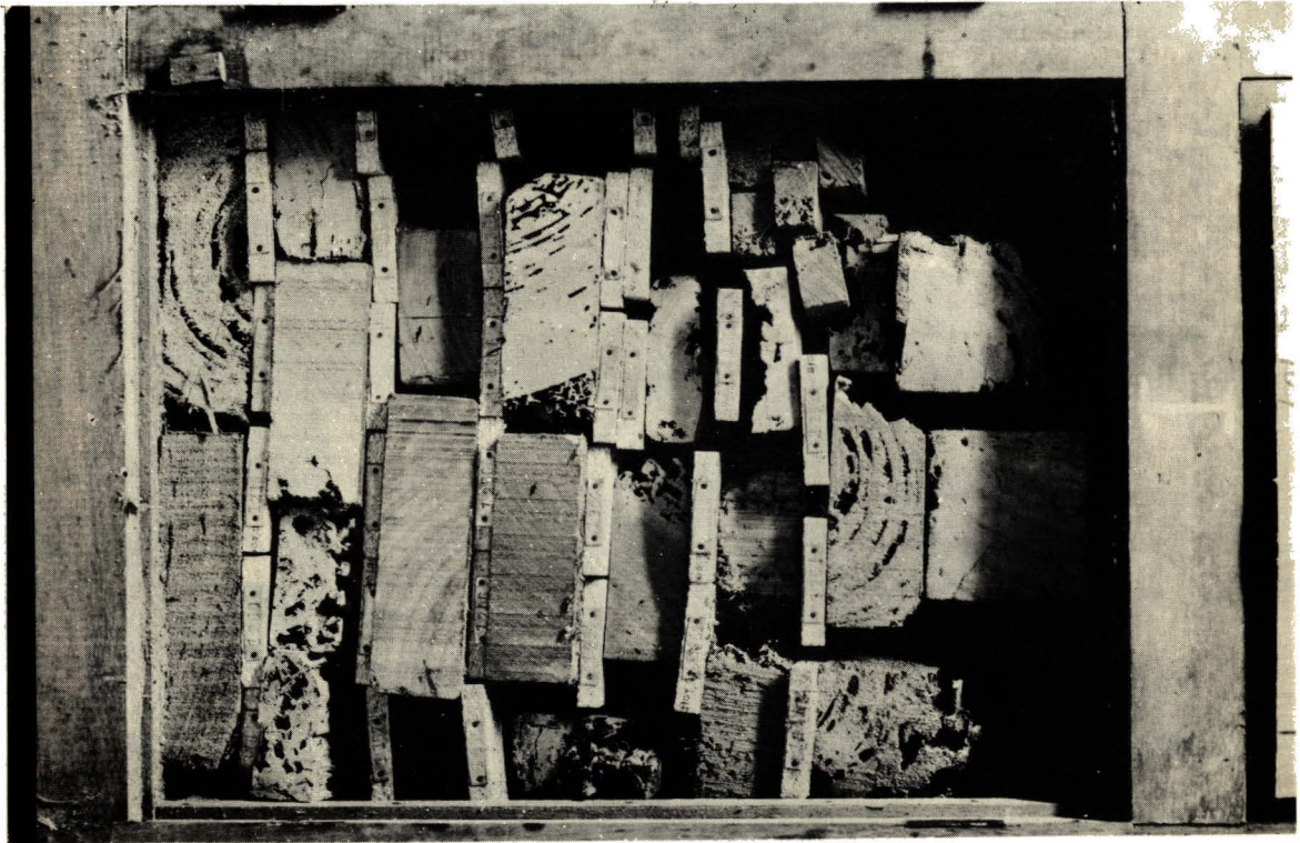
FIG. 2.—Chipboards exposed to C. cyanocephalus Light, a drywood termite species, in a compartment of a screened cage in the F.P.R.I. insectary.
