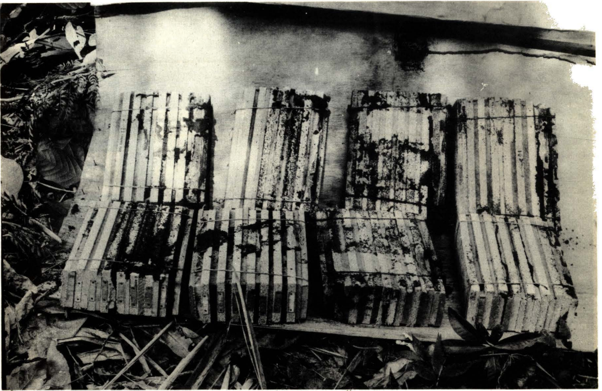
FIG. 1.—Representative bundles of chipboard exposed to subterranean termites, showing the manner chipboards were sandwiched by white luan ( Pentacme contorta (Vid.) Merr. & Rolfe) boards of same size.
