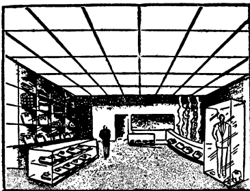
Luminous Ceiling Lighting
