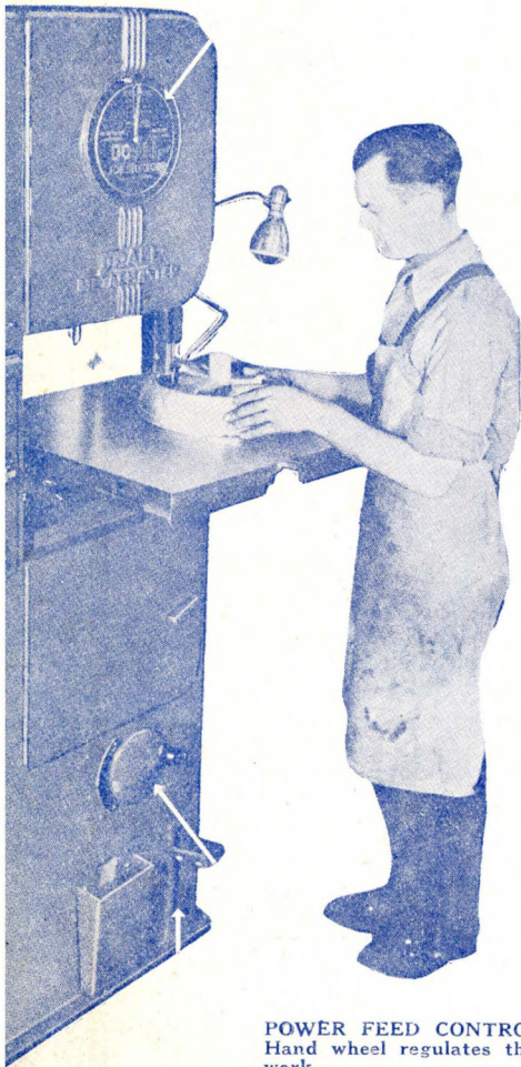
POWER FEED PEDAL Instantly releases all pressure on the work.
