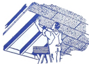
Lay Canec underneath G. I. Roofing to keep out heat
