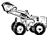
Hough Payloader 1/2 to 3 cu. yd. bucket capacity. Dies, loads, levels, backfills, spreads, lifts, lowers, pulls and pushes.
