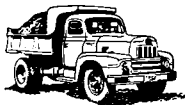
Model R-160 (4x4) Dump Truck. 172-inch wheel base. Power take-off openings for auxiliary equipment.
