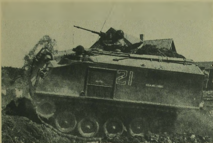
The armored personnel carrier provides protection from small arms fire as well as from shell fragment while delivering infantrymen and firepower into combat areas.
