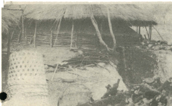
Figure 3. Showing a country-side charcoal kiln (Japanese style beehive type) taken outside of Taipei. It takes about 2 weeks to convert the green wood of Acacia confusa into charcoal in this type of charcoal kiln.
