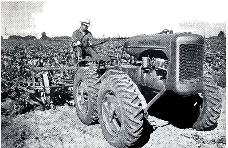
EIMCO Power-Horse pulling horse-drawn-type cultivator in beet-sugar field.
