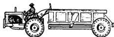
Model 2T-75, 2-wheel Rubber Tired Tractor and 2W-75 Bottom Dump Wagon. Heaped Capacity 20 cu. yd.
