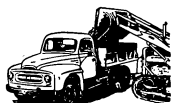
R-164 Series, International Dump Truck. Gross Vehicle Weight, 17,000 pounds; Body dimensions in inches: 108x78x15. Proved steel-flex frame. Wide variety of trucks and dump bodies available.
