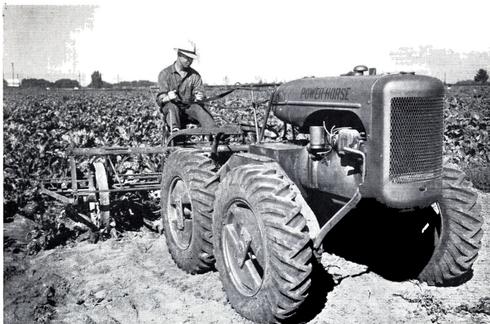
EIMCO Power-Horse pulling horse-drawn-type cultivator in beet-sugar field.
