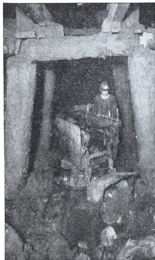
Loader operating in narrow drift
