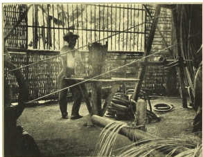
Operator drilling seat piece.
