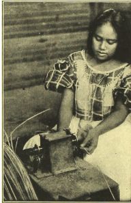
Making rattan splits of uniform width.
