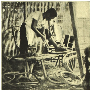
Fastening the ends of seat piece.
